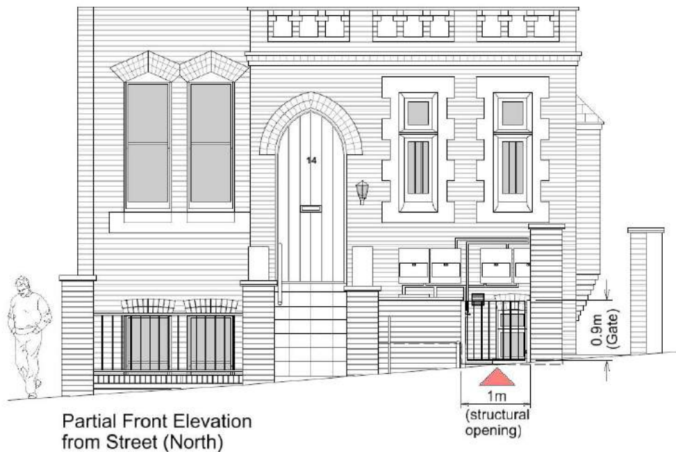
Image 12 – Proposed front street elevation of external refuse storage area. Image taken from architectural drawing ref: 'A22012 A(S3)05 – Proposed Plan, Front Elevation, Sections' (Not to scale).
