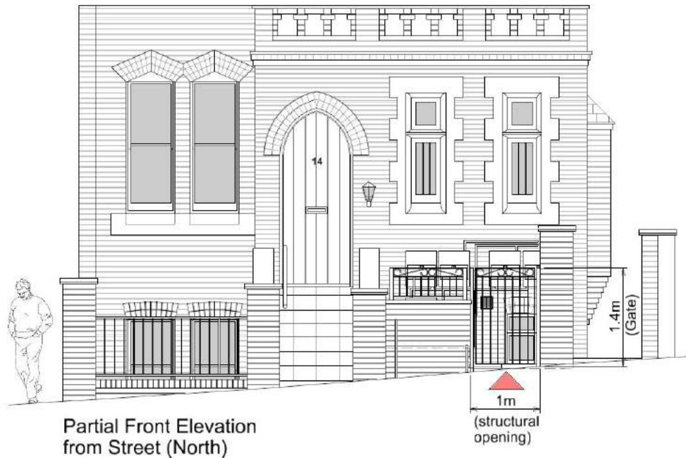
Image 11 – Previously proposed front street elevation of external refuse storage area, presented at pre-application advice stage. Design now superseded by the submitted design proposal shown within Image 12 below (Not to scale).
