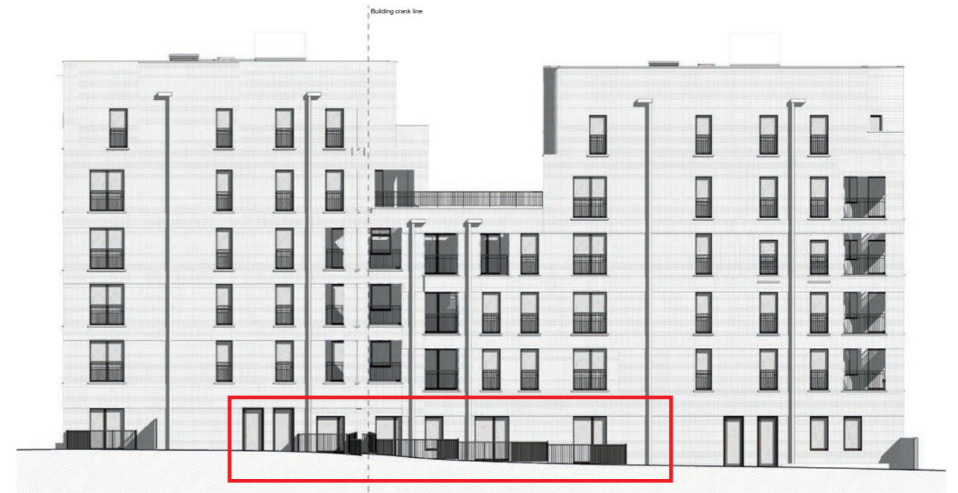
Block I, Proposed west elevation, changes clouded in red. Drawing: AGV-HBA-I-ZZ-DR-A-200200_P3
