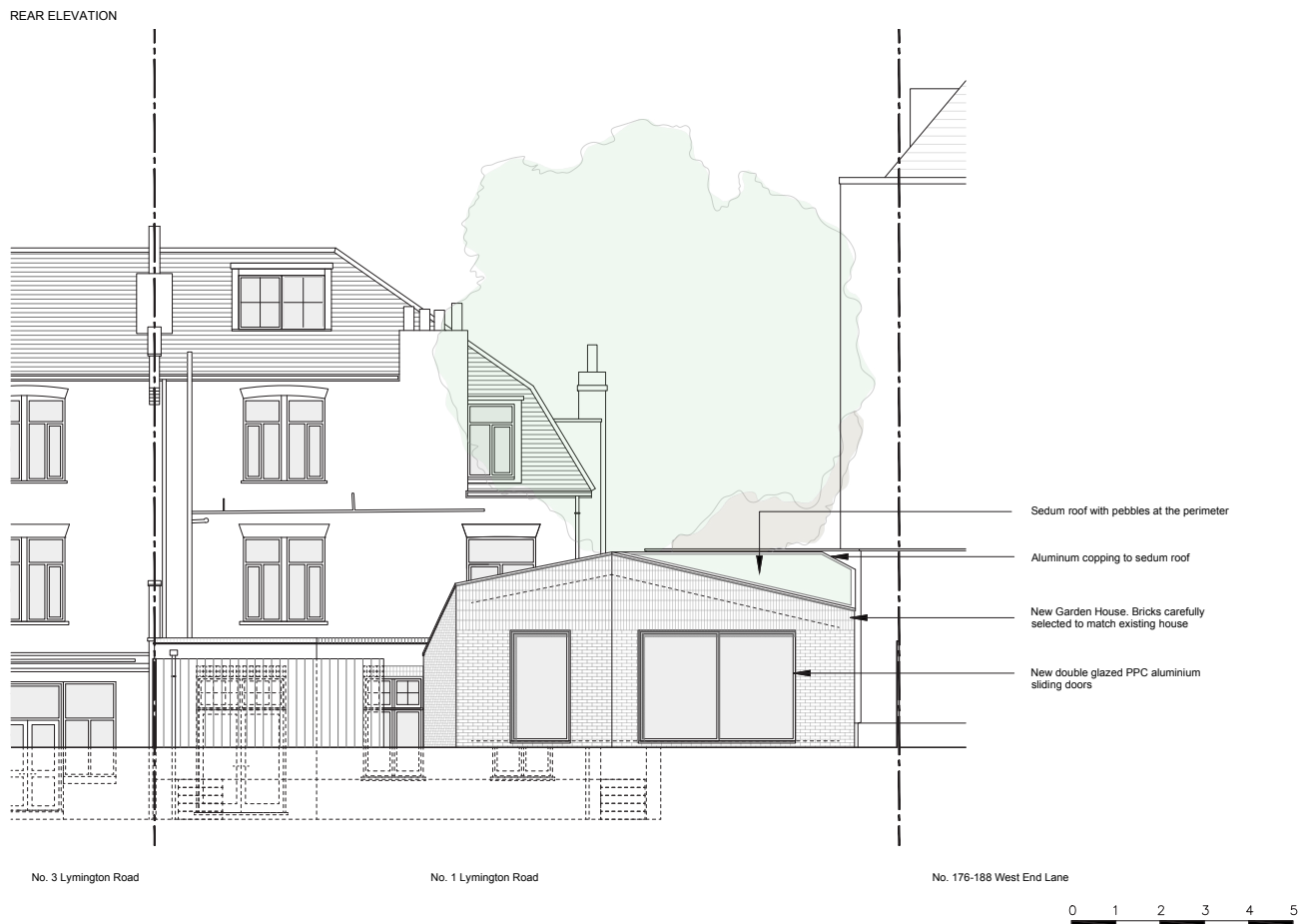
Rear elevation drawing showing the proposed new dwelling house, the gently pitched roof form echoing the distinctive double pitched roof to the host building.
