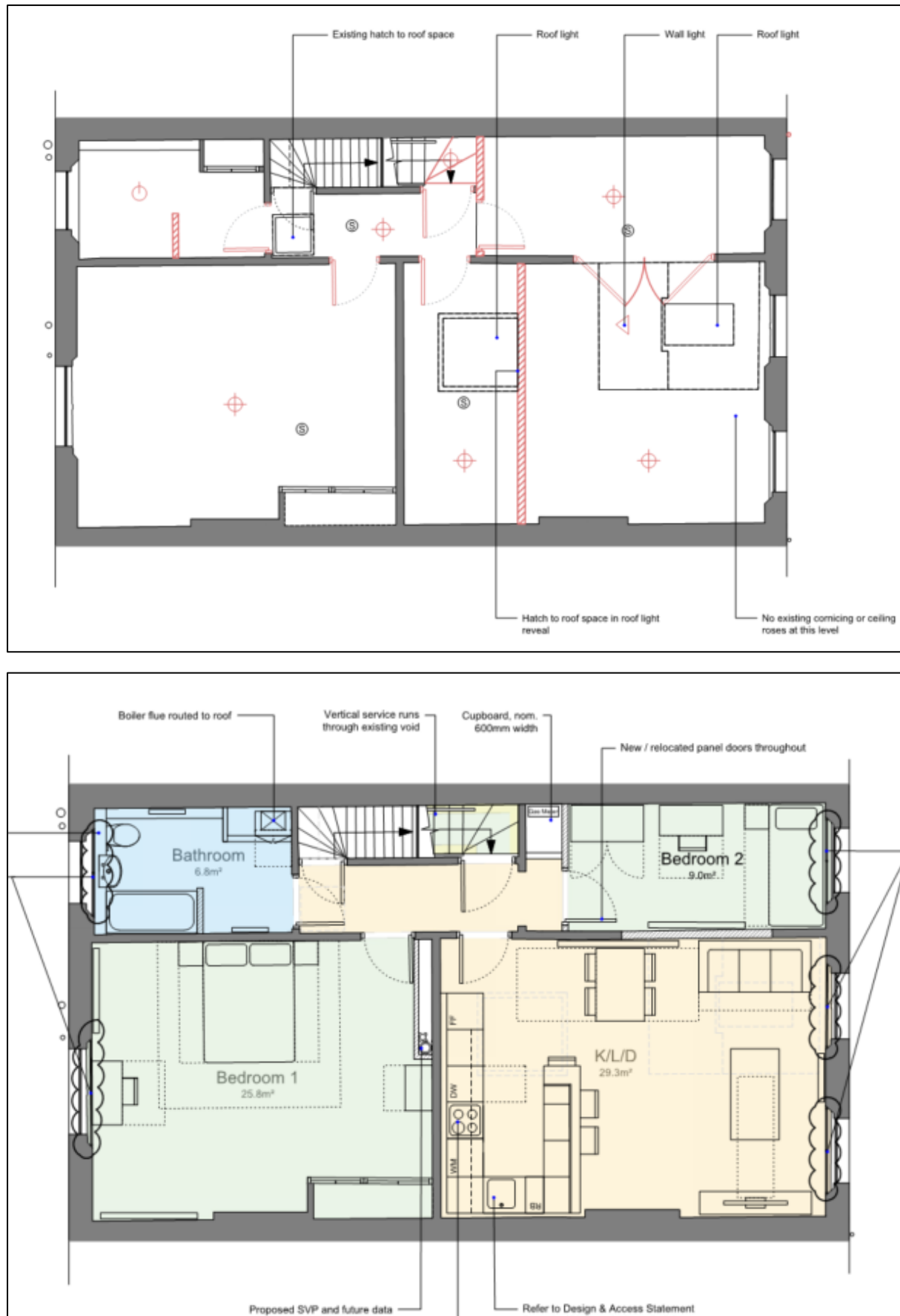
Fig 6. Existing (top) and proposed (bottom) third floor plan.
