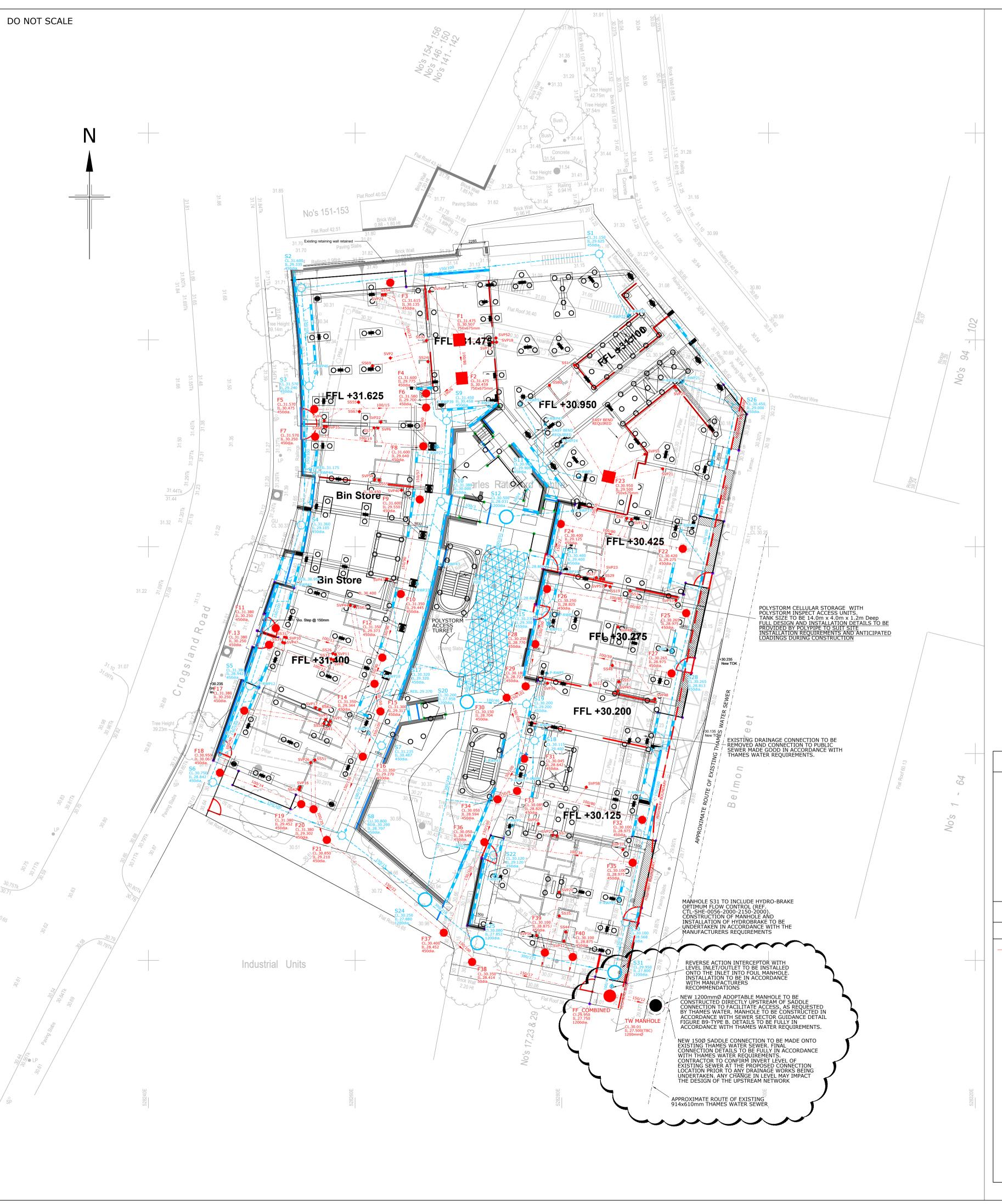
THE SURFACE WATER DRAINAGE DESIGN HAS BEEN BASED UPON THE STANTEC FLOOD RISK ASSESSMENT REF. 43006, DATED JULY 2020 WHICH PROPOSES A MAXIMUM SURFACE WATER DISCHARGE OF 2 LITRES/SECOND FOR ALL STORM EVENTS UPTO AND INCLUDING THE 1 IN 100 YEAR + 40% CLIMATE CHANGE EVENT.
