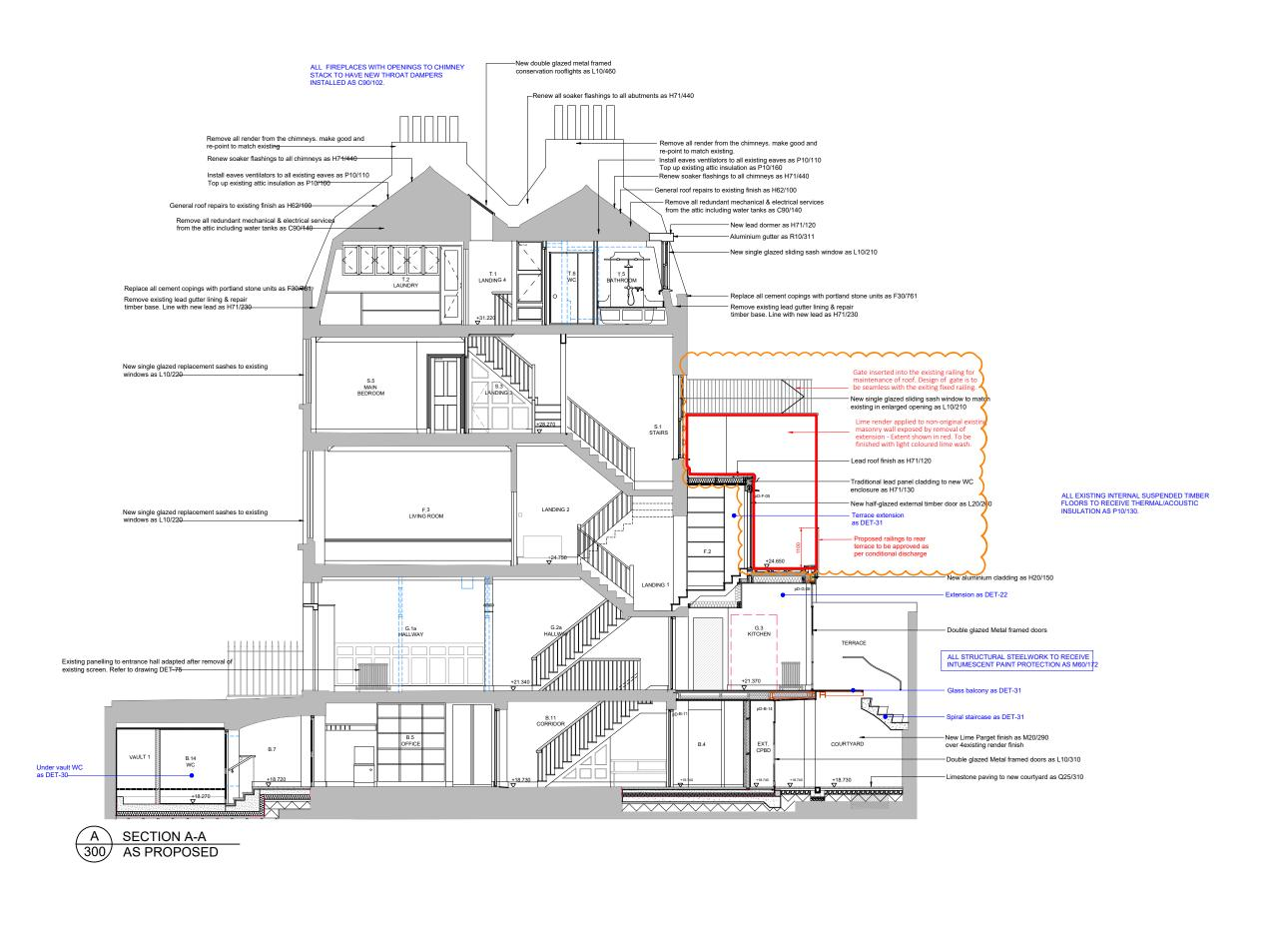
DO NOT SCALE DRAWINGS. THE CONTRACTOR IS RESPONSIBLE FOR CHECKING DIMENSIONS ANY DISCREPANCY IS TO BE REFERRED TO TI ARCHITECT. Lime render specification: part NHL 3.5 Lime 2.5 parts 0/4 sharp sand Polypropylene fibres Top coat 1 part NHL 3.5 Lime 2.5 parts 0/4mm sharp sand PLANNING December 23 PLANNING August 21 PLANNING May 21 DATE REV. AMENDMENT THOMAS & PARTNERS
