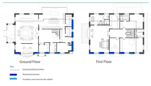
Figure 7: Key plan, proposed Refurbishment & Extension option
