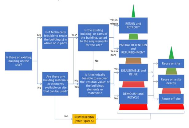
*Figure 5: Decision tree for design approaches for existing structures/buildings (Source: GLA Circular Economy Guidance)*
