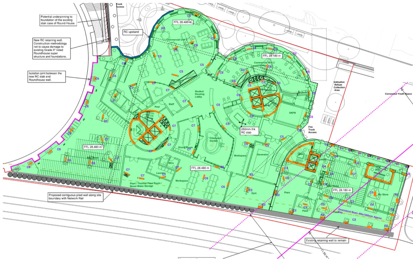
Figure 31 - Proposed ground floor plan showing the extent of the proposed contiguous piled wall.
