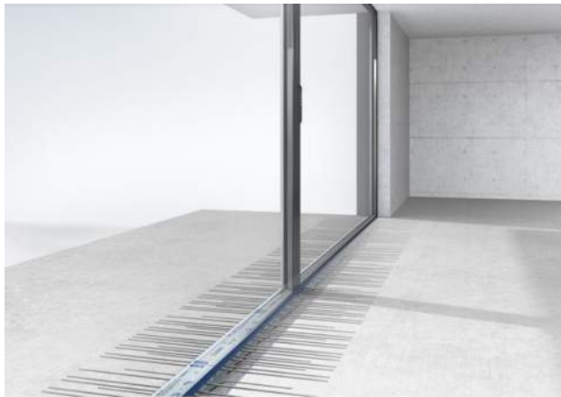
Figure 25 - 3D Image of concrete cantilever with thermal break
