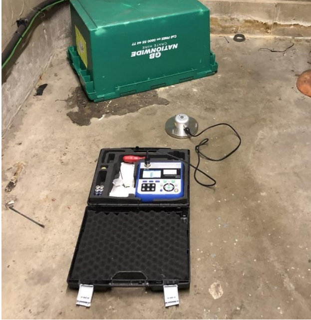
Figure 8 Internal vibration measurement position V
