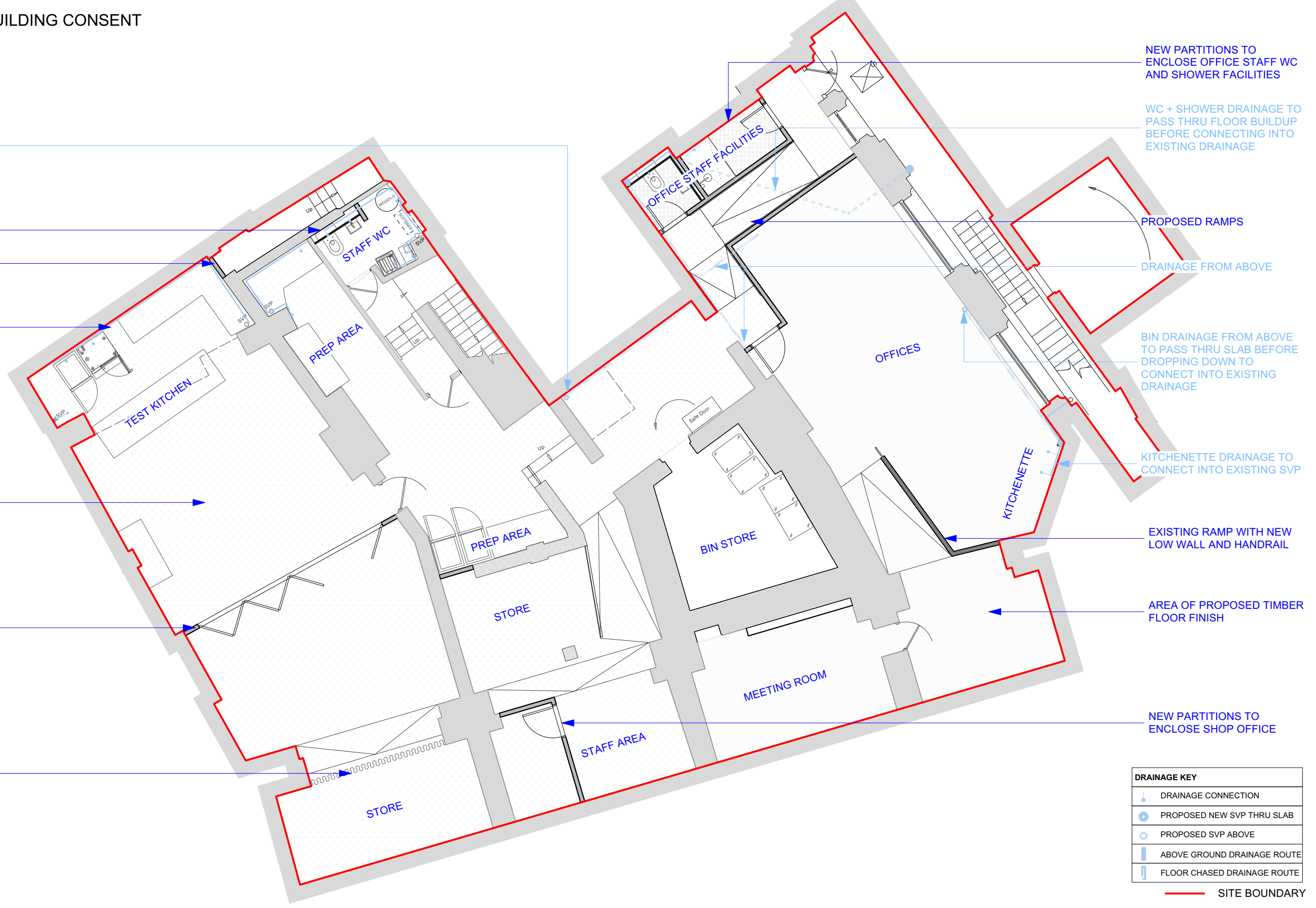
01 PROPOSED BASEMENT PLAN Scale: 1:100
