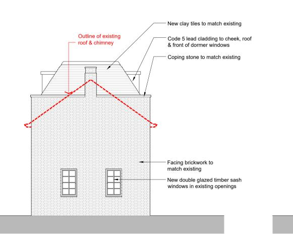
PROPOSED SIDE (NW) ELEVATION Scale 1:100 @ A1
