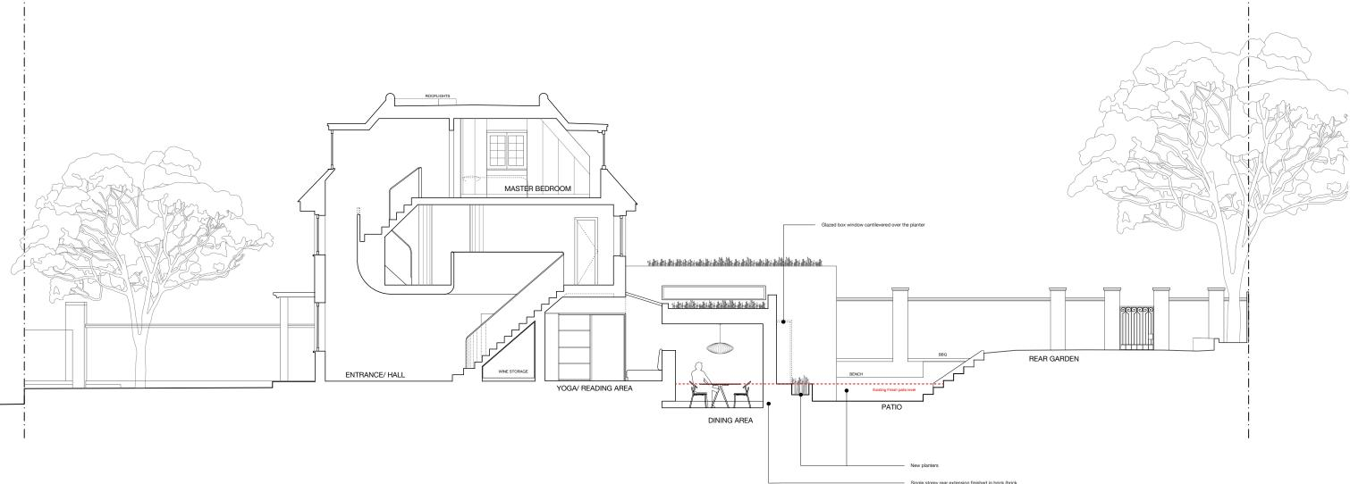
Single storey rear extension finished in brick (brick colour to match the existing) with green roofs. Sunken extension with respect the existing ground level
