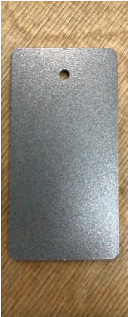
MS light fixtures to be finished in RAL820M Silver to match LWL bead blasted steel.
