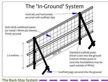
This system will be installed where indicated by a dashed purple line on the Tree Protection Plan. It is more practical over existing hard surfaces or where the fencing needs to be moved to enable permitted activities within a Restricted Activity Zone. This system is able to withstand occasional knocks by machinery and must not be relocated except with the consent of the site manager and the approval of the local authority.
