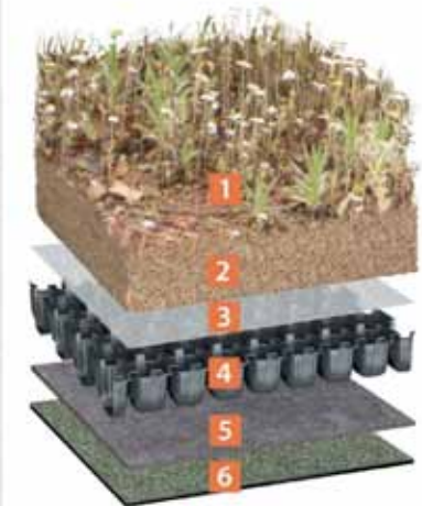
Indicative extensive green roof system - seeded
