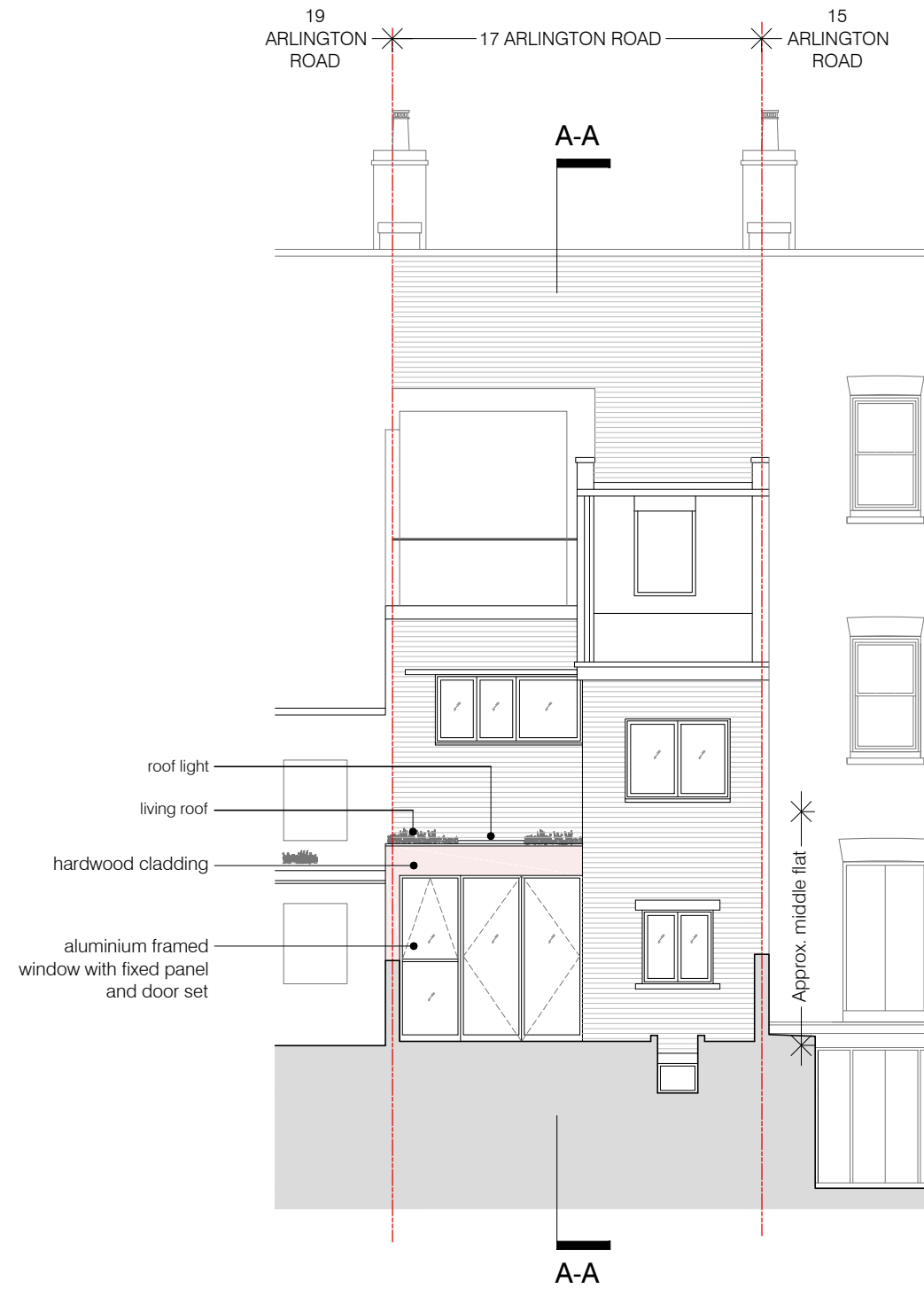
01 PROPOSED REAR ELEVATION scale 1:100
