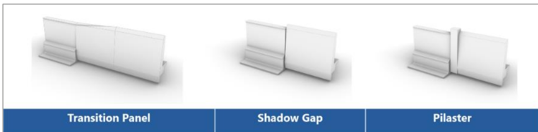
Figure 22 Initial parapet transition options
