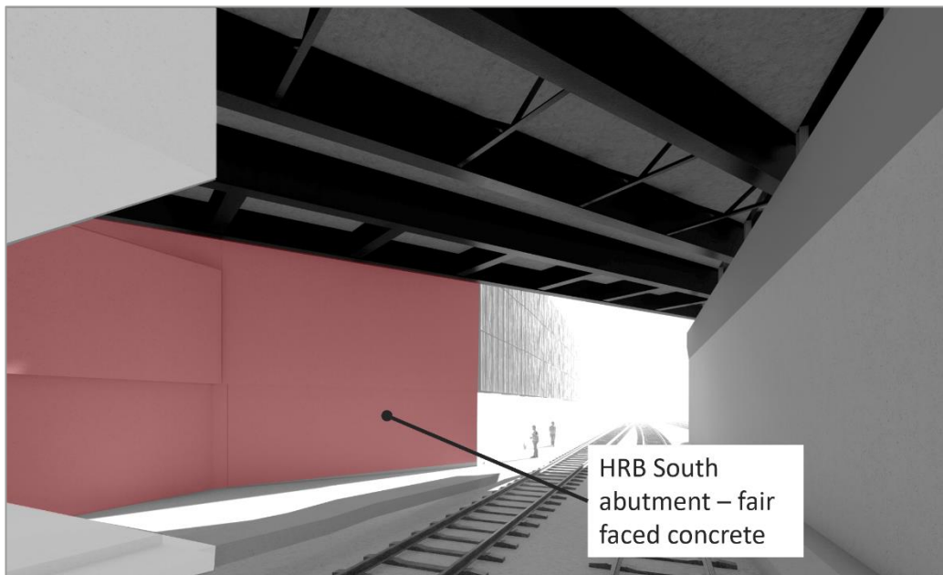
Figure 20 Proposed lining wall at the south abutment
