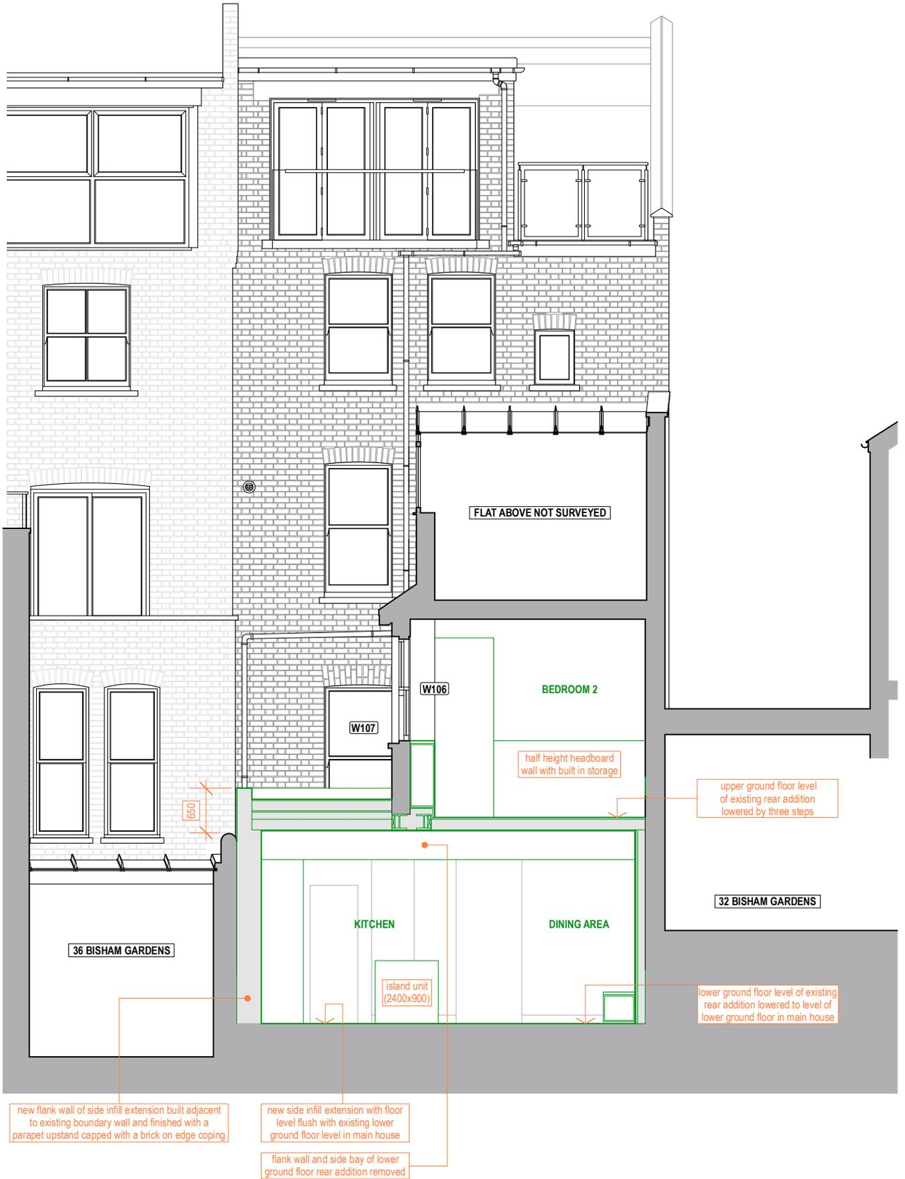
new flank wall of side infill extension built adjacent to existing boundary wall and finished with a parapet upstand capped with a brick on edge coping
