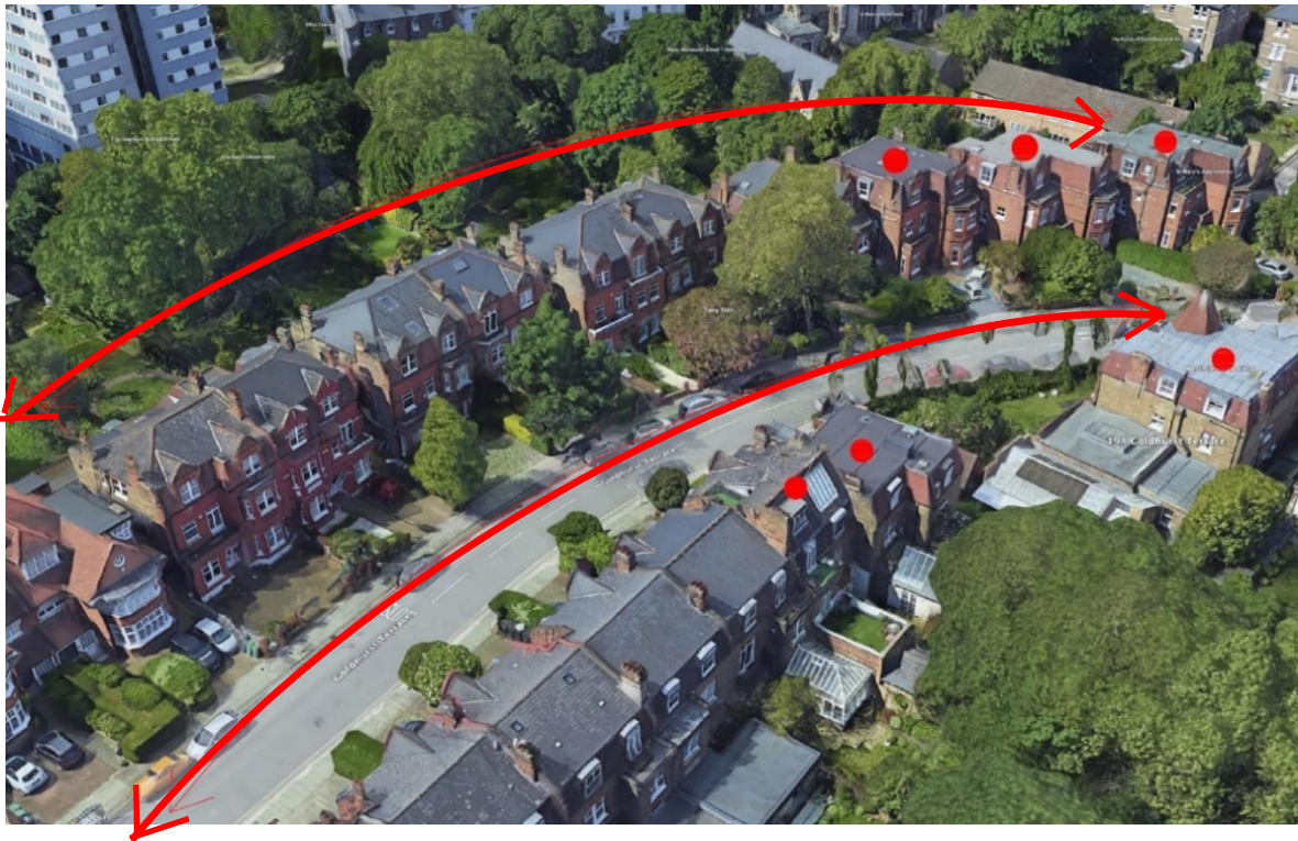
Figure 8. Aerial view of roofscape from North East. The red arrows indicate the building that form part of the same group as No194, and the red dots the buildings whose roofs are considered to have been rebuilt.
