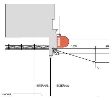
The Design CPG states that confirms that awnings should be retractable, of traditional canvas, have the blind box integrated into the design, be attached between the shopfront and fascia, of a width appropriate to the shop front and be flush with the fascia level.
