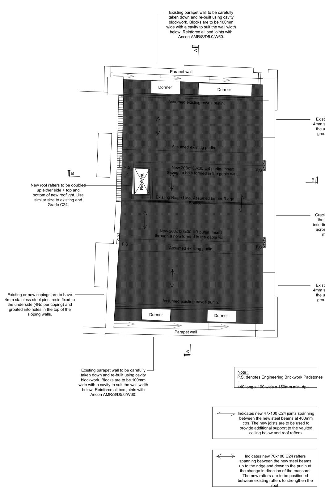
Existing or new copings are to have 4mm stainless steel pins, resin fixed to the underside (4No per coping) and grouted into holes in the top of the sloping walls.
