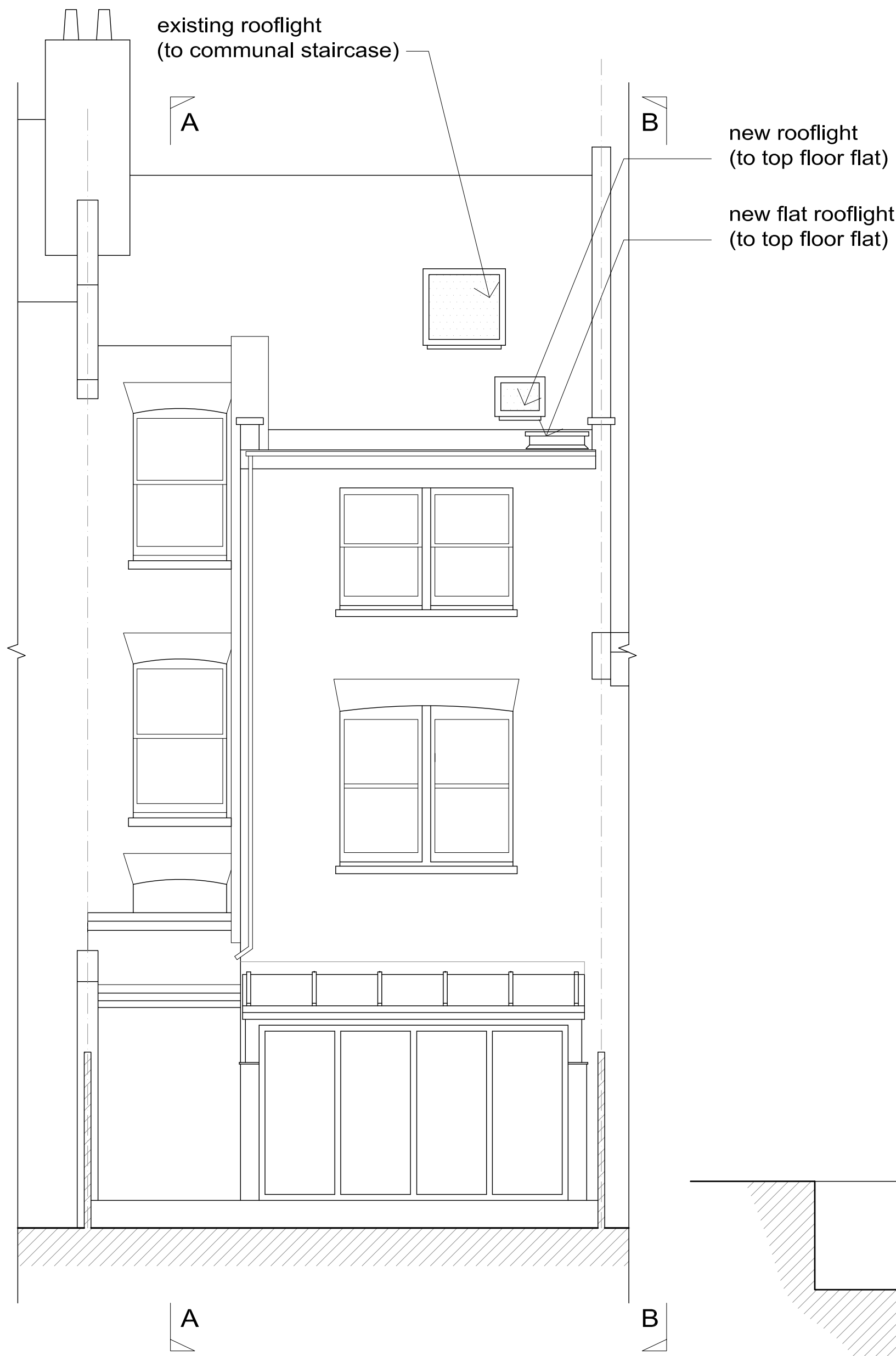
West elevation (to rear)
