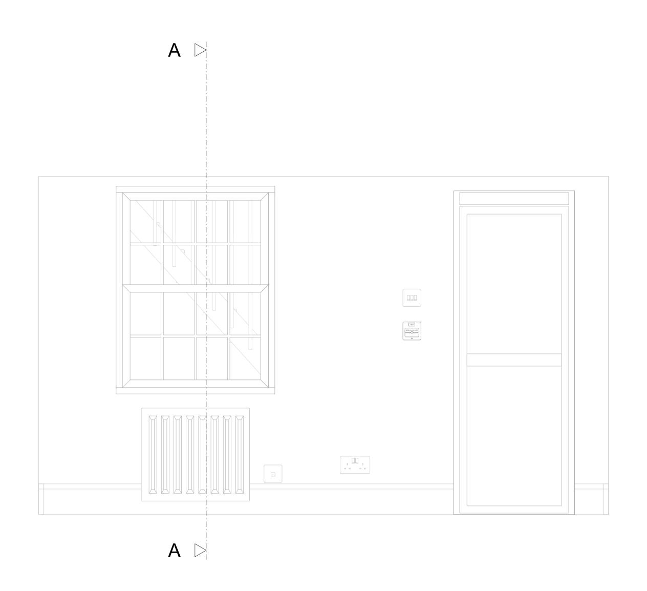
**FRONT** Internal Elevation Scale 1 : 25
