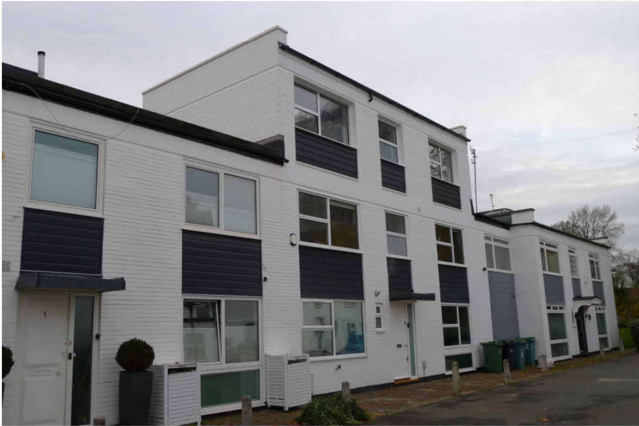
Numbers 1 and 2 Lyttleton Close, Front elevation. Alternative window designs, double casements at number 1. No2 has windows divided into 3 parts with a opening top vent.
