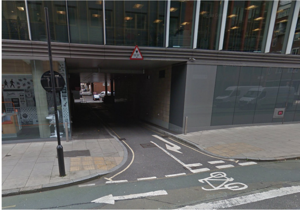
Figure 4.3: Existing Height Restriction for Waste Vehicle Access
