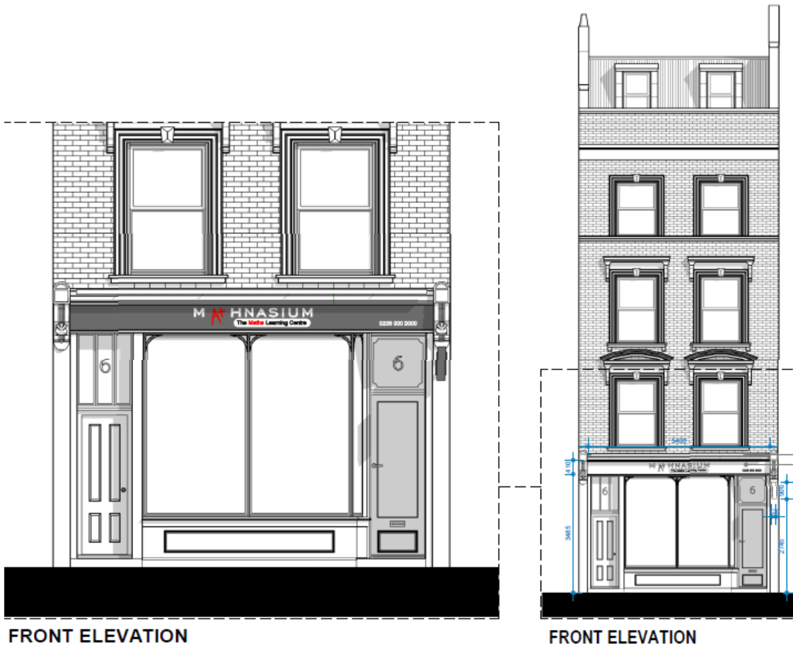
Figure 5: Proposed Front Elevation.
