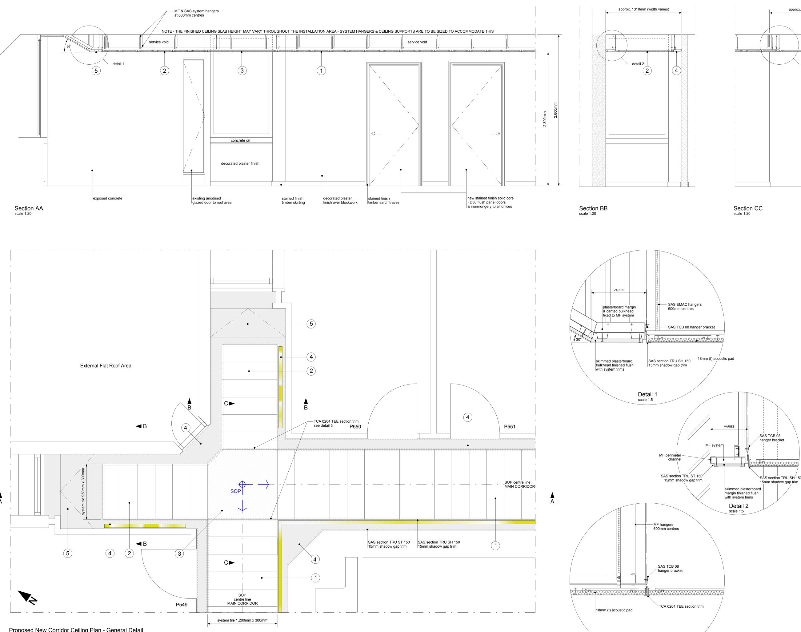
Proposed New Corridor Ceiling Plan - General Detail scale 1:20
