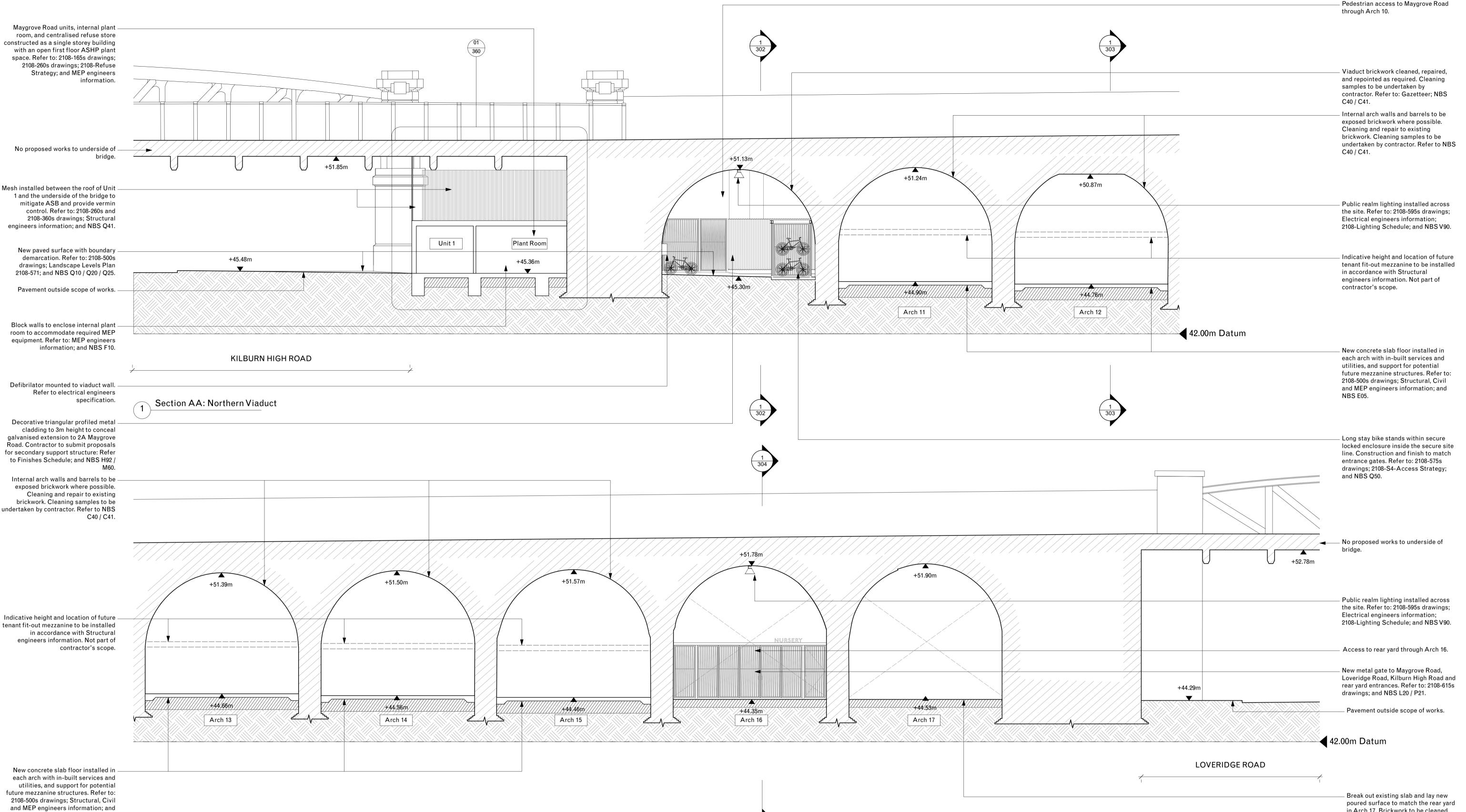
New concrete slab floor installed in each arch with in-built services and utilities, and support for potential future mezzanine structures. Refer to: 2108-500s drawings; Structural, Civil and MEP engineers information; and NBS E05.
