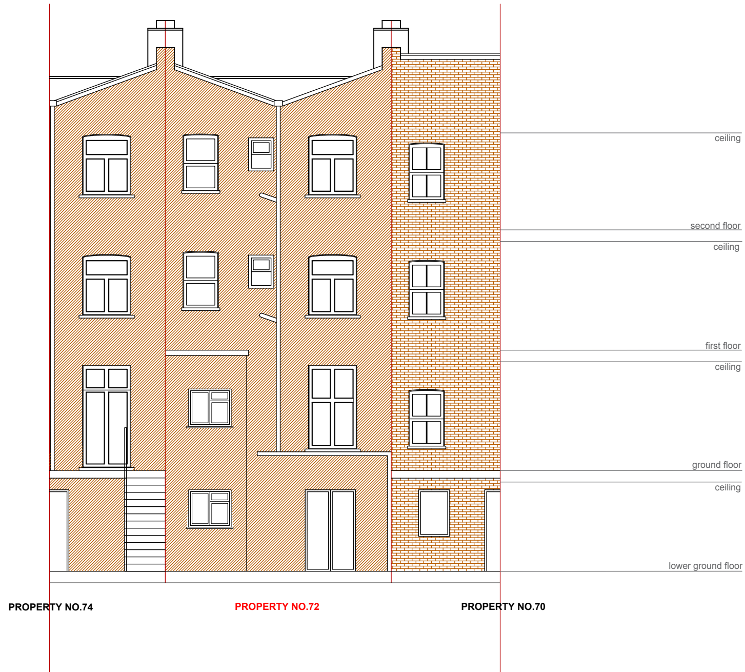
12 REAR ELEVATION - EXISTING 1:100 @A3
