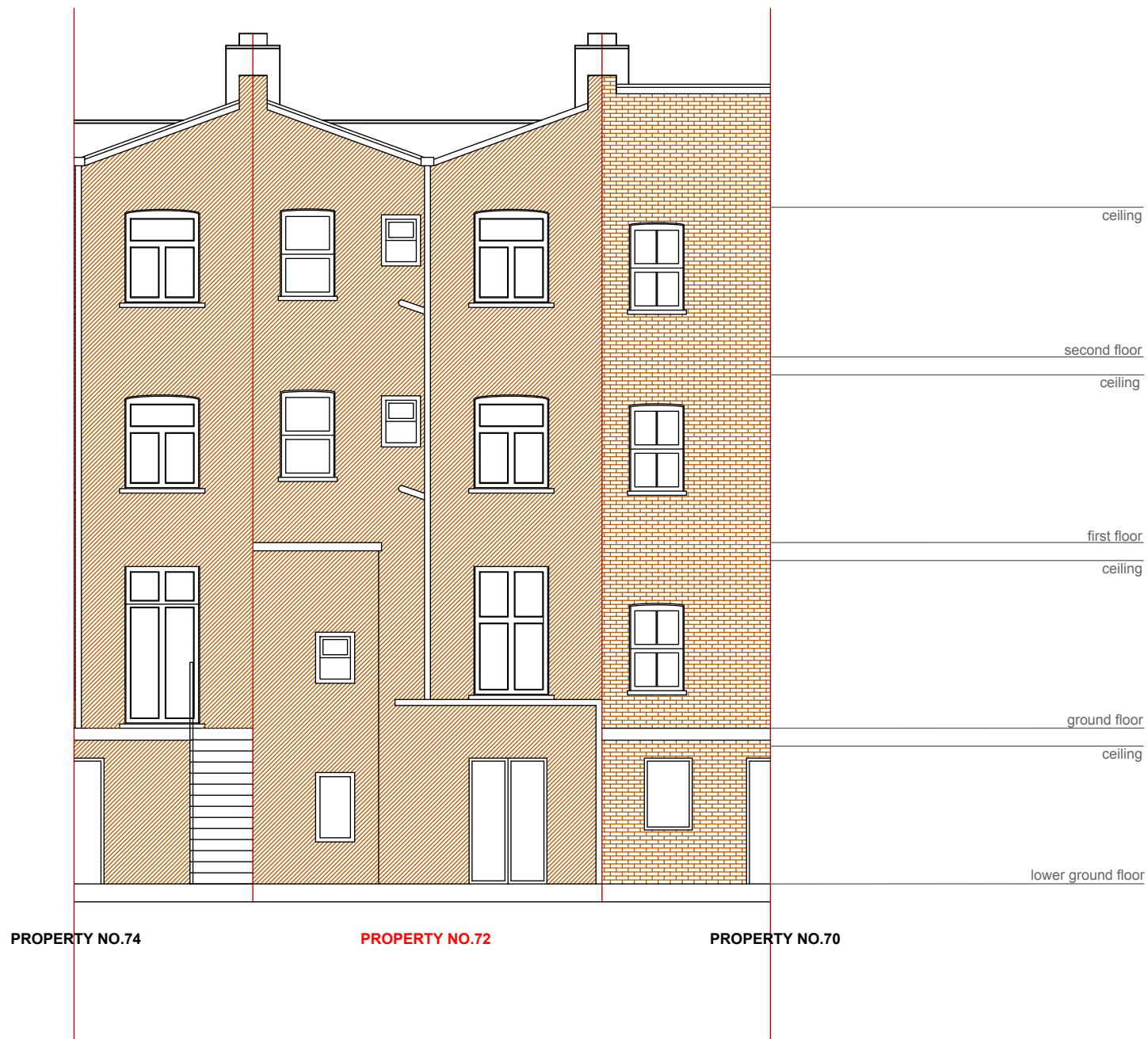
13 REAR ELEVATION - EXISTING 1:100 @A3
