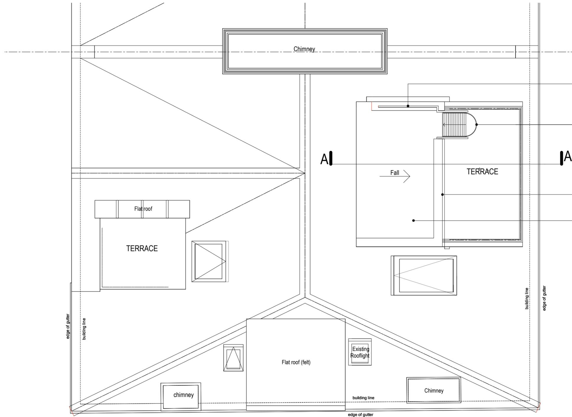
New safety railing - height 1100mm from flat roof - between access ladder and chimney breast (location of TV aerials).
