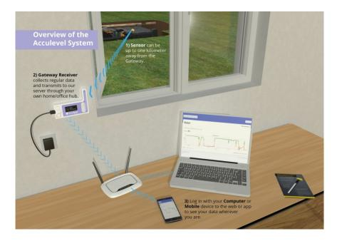
The Rain Acculevel will accurately measure the water level in your rainwater tank giving readings that you can view on a PC or smart device. Using the latest wireless technology it works on tanks below or above ground and over long distances.
