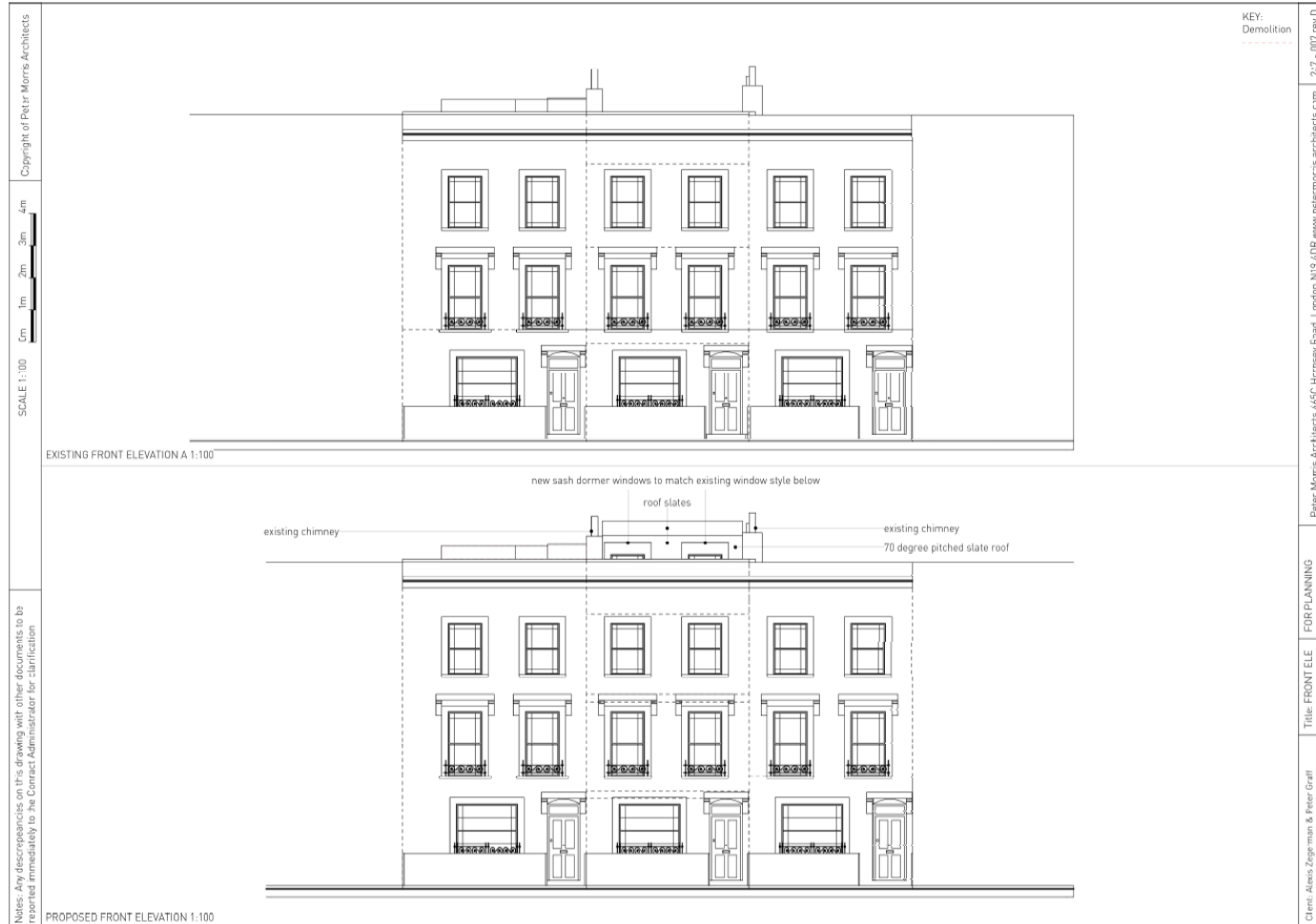
Figure 18: Existing (top) and Proposed front elevation – note the mansard will not be visible from the streetscape.
