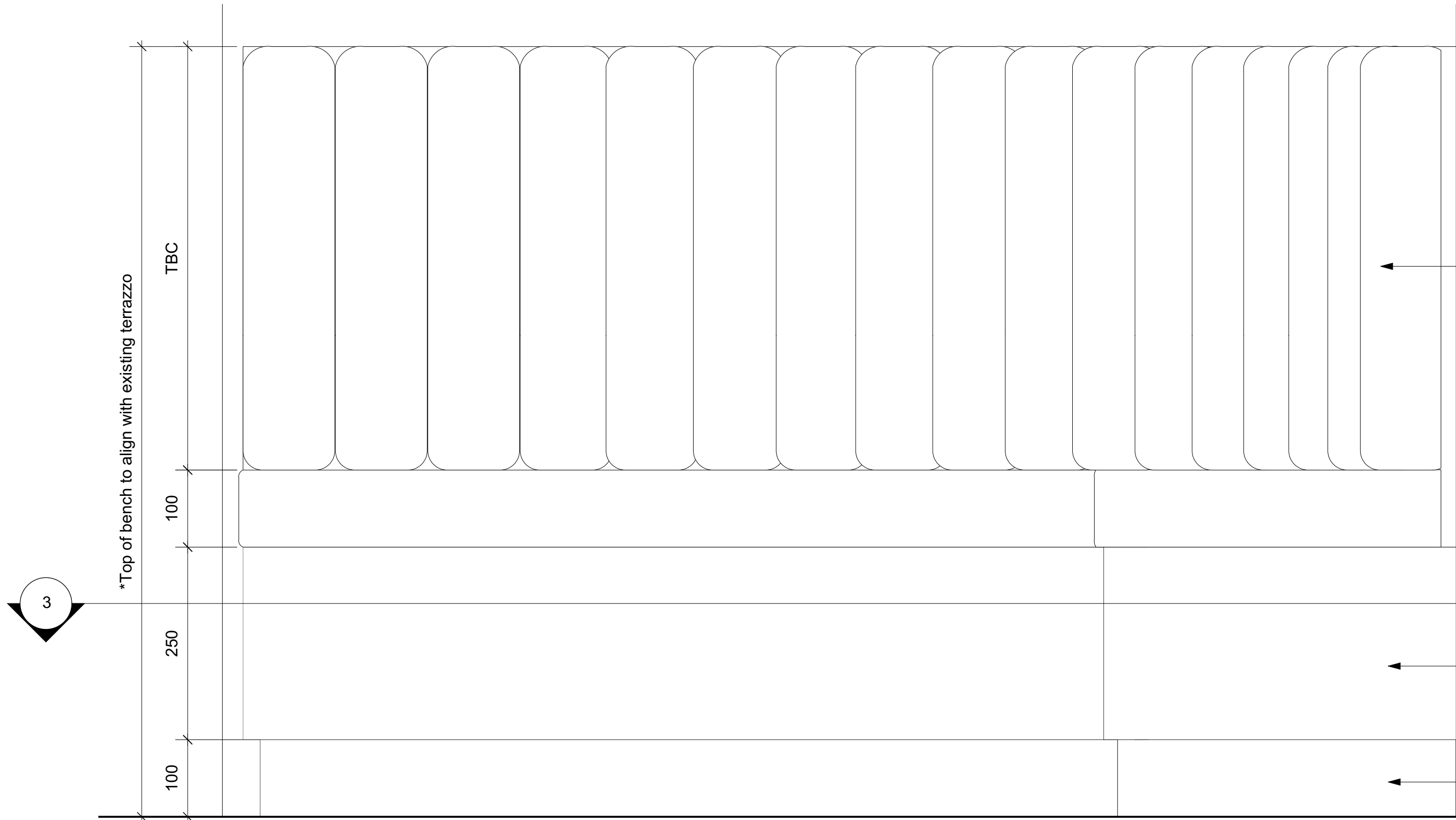
2 Reception Bench Elevation Scale: 1:5
