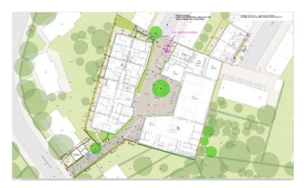
The lower 300 mm of the 750 mm thickness installed in the soft landscaped areas to the north and south of Block A and the West of Block D comprised clean imported 6F5 and Type 1 MOT material, creating a boundary layer between the underlying soil and the imparted material, deterring future excavations. Therefore a membrane, as detailed in the remediation method statement, was not installed. A 450 mm thickness of clean imported topsoil was then installed above.
