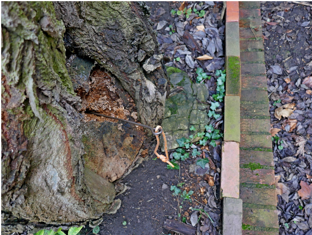
2) Steel probe in decaying wound at the base of tree 19. This went in 400mm with minimal resistance.
