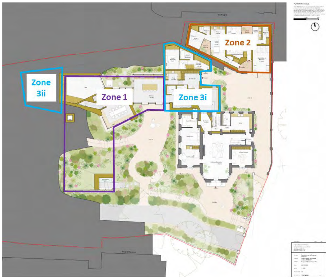
Figure 2.3 First floor plan, annotated with the three zones of proposed development (red line indicative of site boundary)
