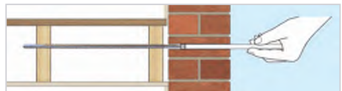
3. Fit the plastic sleeve over the BowTie HD and use the support tool to push it to the back of the hole in the wall (outer leaf in a cavity wall)
