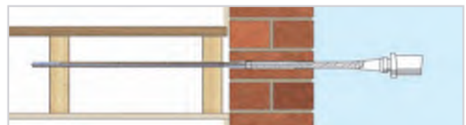
4. Inject PolyPlus resin to fill the hole and bond the BowTie HD to the masonry, allow the resin to gel and then make good
