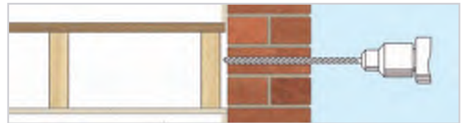
1. Mark the position of the joist centre on the external wall and then drill a clearance hole (normally 16mm) through the wall. Clean out the hole
