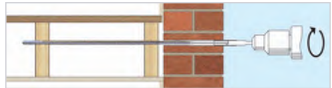
2. Fit the BowTie HD Support Tool to an SDS rotary hammer drill, insert the BowTie HD and drive it (off hammer) into, and through, the first and second joists
