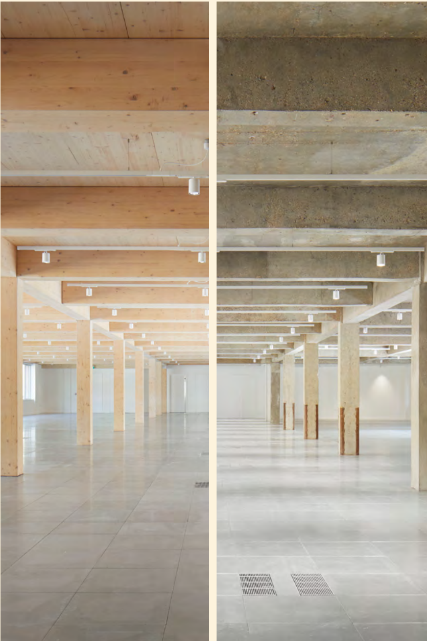
By retaining 85% of the existing building structure we are able to dramatically reduce the embodied carbon of the building vs. a demolition and new build.
