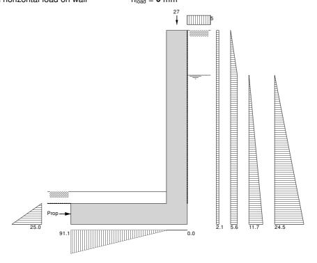
Loads shown in kN/m, pressures shown in kN/m<sup>2</sup>
