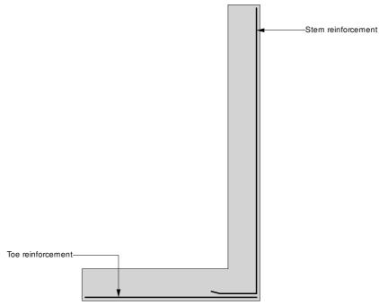
Toe bars - 16 mm dia.@ 150 mm centres - (1340 mm²/m) Stem bars - 16 mm dia.@ 150 mm centres - (1340 mm<sup>2</sup>/m)
