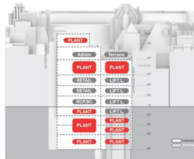
Schematic cross section showing the spatial distribution for the required plant equipment at Furnival Street.
