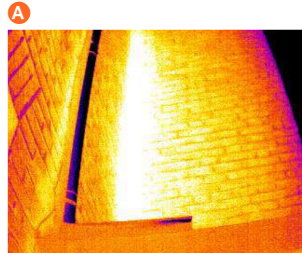
A Heat loss from uninsulated walls at rear of house
