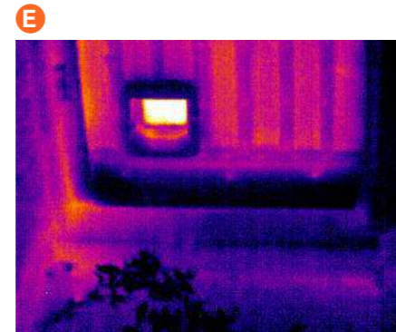
E Heat leaking through the back door is so severe that the thermal camera reveals the timber stud door structure. Note also the severe heat loss from a leaky cat flap. A Passive House cat flap will eliminate this problem.
