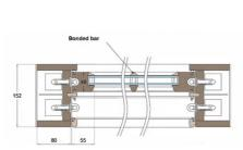
D Loc - section through jamb and stiles
