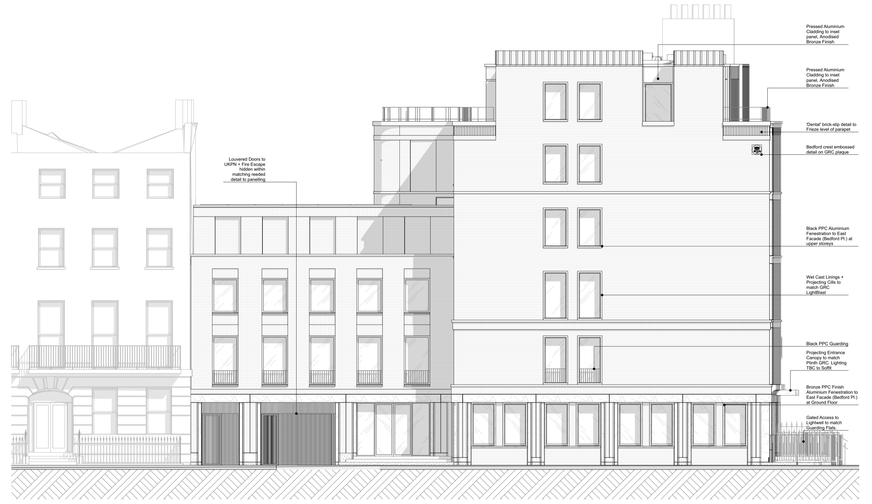
E East (Bedford Place) Elevation 1:100
