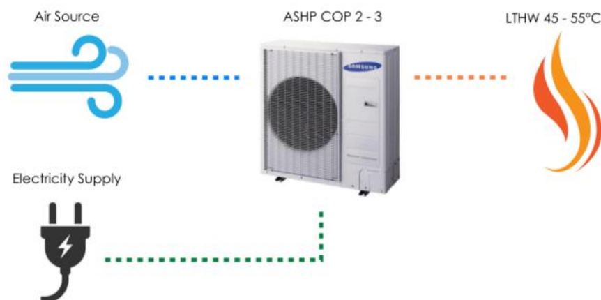
Figure 1 - Simplified diagram of an air source heat pump system. Values of COP typically range from 2-3 for an ASHP delivering 45-55°C LTHW. Note that most models have a secondary mode to generate higher temperatures for domestic hot water, with a commensurate reduction in COP.
