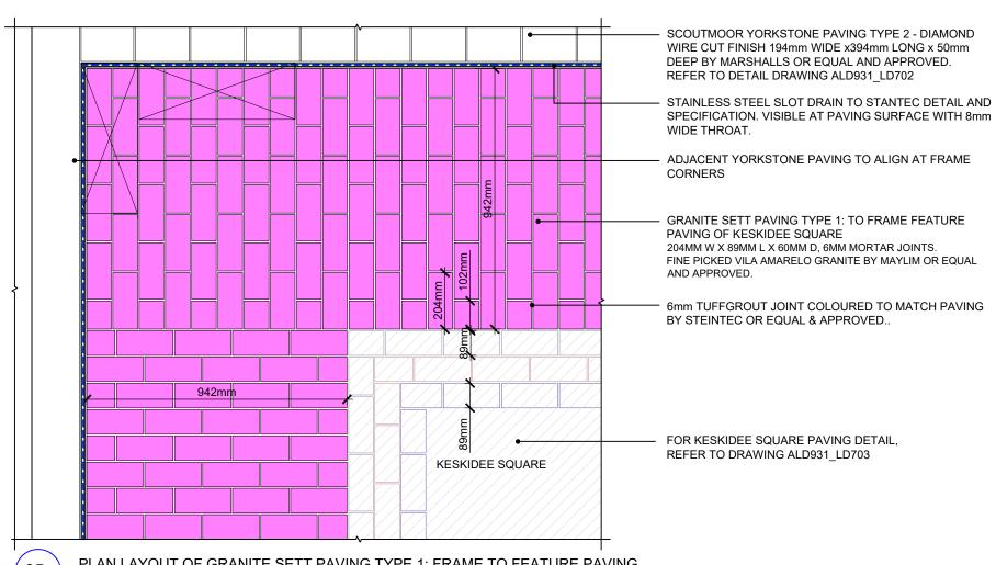
PLAN LAYOUT OF GRANITE SETT PAVING TYPE 1: FRAME TO FEATURE PAVING 05a SCALE: 1:15 @ A3
