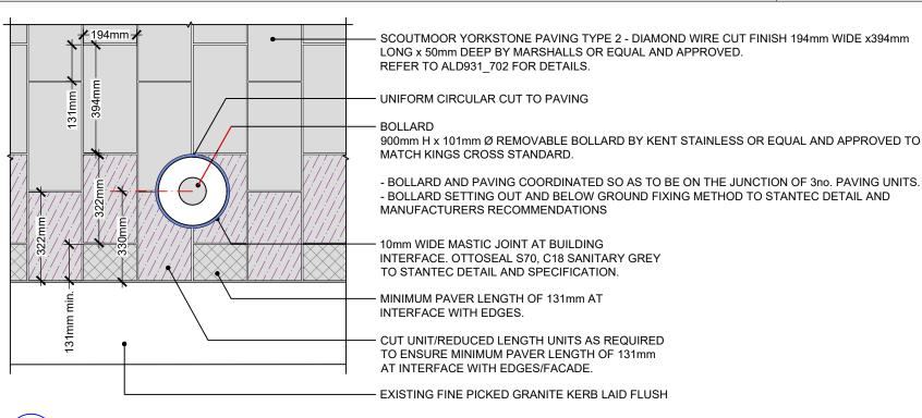
DETAIL PLAN OF REMOVABLE BOLLARD INTERFACE WITH YORKSTONE PAVING (DETAIL ILLUSTRATED AT JUNCTION WITH S1 AND S2) SCALE: 1:15 @ A3
