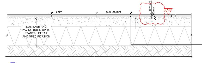
SCOUTMOOR YORKSTONE PAVING TYPE 1a/b - DIAMOND WIRE CUT FINISH 600 mm WIDE x  $600 \hbox{-} 900 mm$  LONG x 50 mm DEEP BY MARSHALLS OR EQUAL AND APPROVED.
