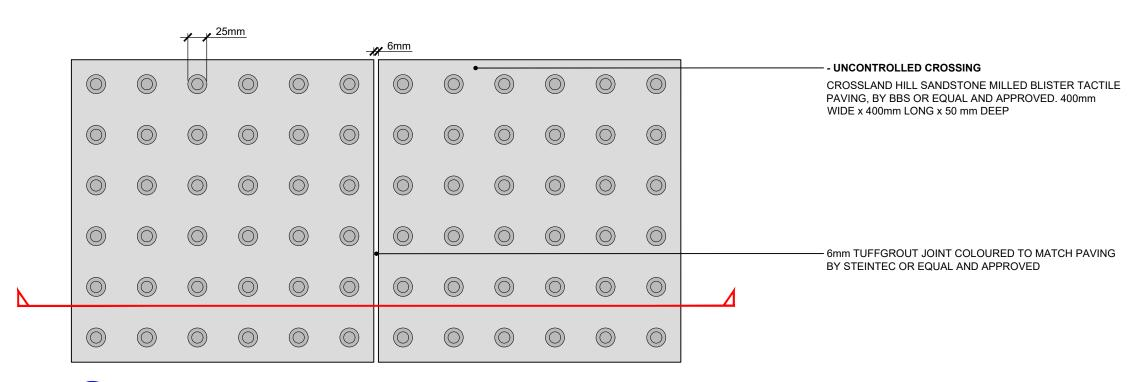
PLAN LAYOUT OF TACTILE PAVING TYPE 1 & 2 SCALE 1:5 @ A3
