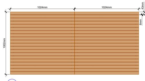
TIMBER BENCH DETAIL PLAN SCALE: 1:15 @ A3
