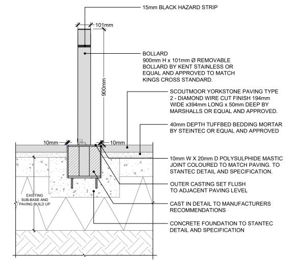
SECTION DETAIL THROUGH REMOVABLE BOLLARD SCALE: 1:15 @ A3
