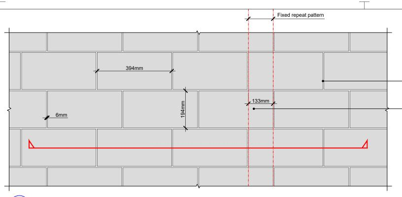
6mm TUFFGROUT JOINT COLOURED TO MATCH PAVING BY STEINTEC OR EQUAL & APPROVED..
