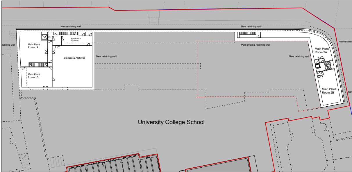
Basement level floor plan after first PreApp stage – with plantrooms and storage / archives space
