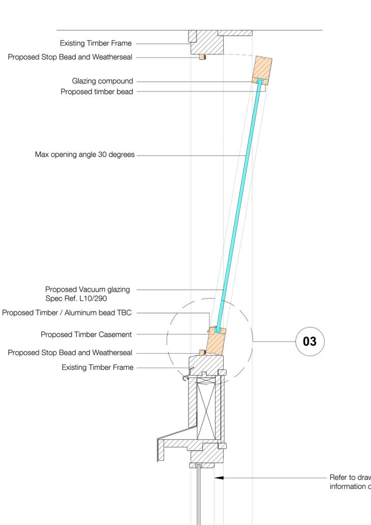
**02 Proposed - Window Vent Head and Sill Detail**
