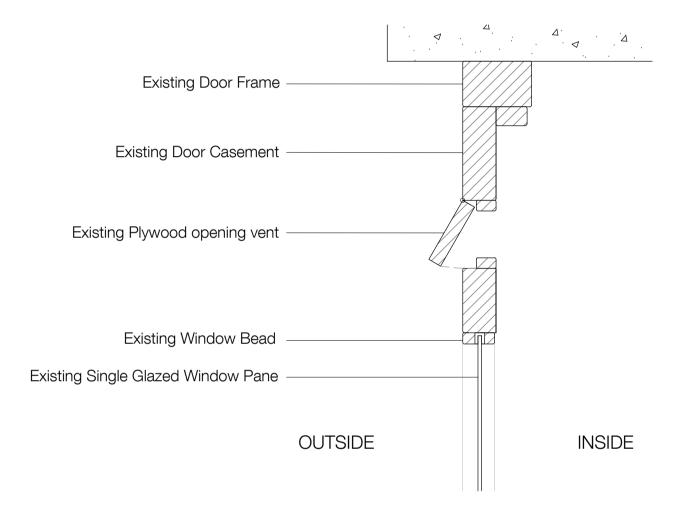
**Existing - Plywood Opening Vent Head - Stable Doors Section Detail**
